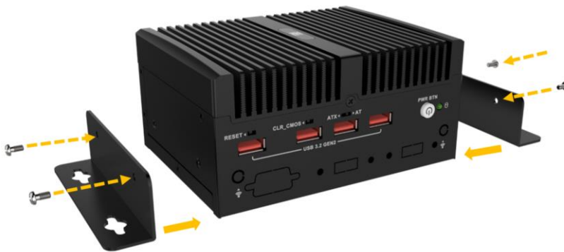
Figure 3-14: Mounting Bracket Retention Screw
