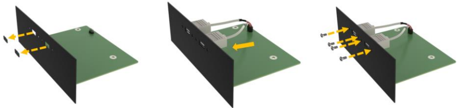
Figure 3-12: USB Cable Type-A Installation
